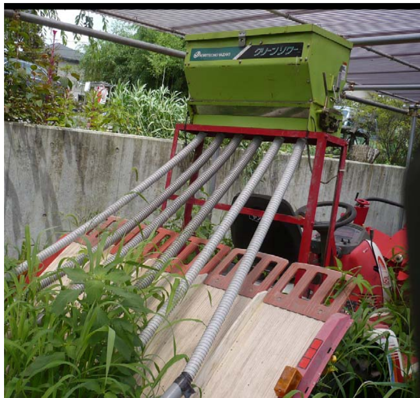
Picture 8: Mr. Inaba's rice transplantation machine with a mechanism that spreads rice-bran pellets evenly (Dominik Rutz, 2007)
